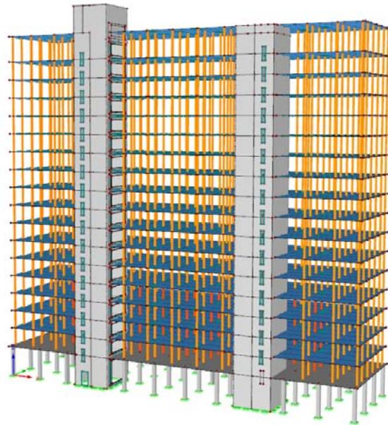
Figure 4: Numerical Model of UBC TWB
