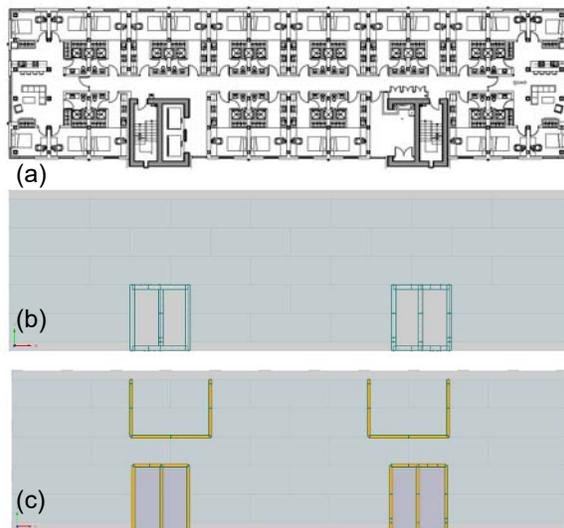
Figure 3: Floor plan of UBC TWB (a); cores for numerical models for designs D2 and D3 (b) and design D4 (c)
