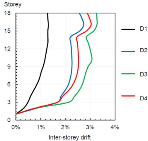
**Figure 6:** Seismic inter-story drift profile for the Y-direction
