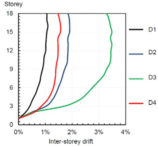
**Figure 5:** Seismic inter-story drift profile for the X-direction
