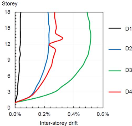
**Figure 8: Wind inter-story drift profile for the Y-direction**
