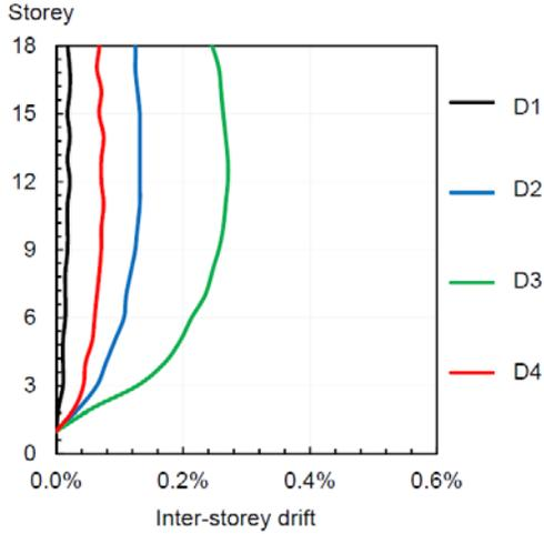
**Figure 7: Wind inter-story drift profile for the X-direction**
