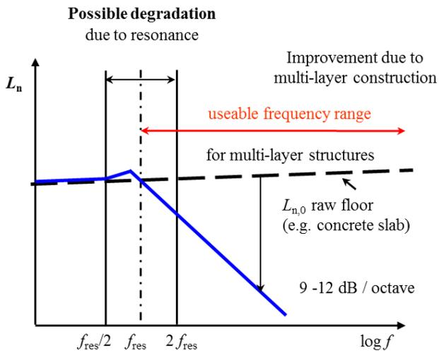
Figure 7: Resonance frequency – multi-layer construction
