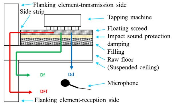
Figure 10: Model of flanking transmission in timber construction Din 4109 (preliminary edition)
