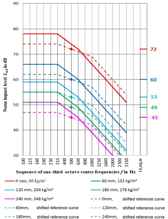
Figure 5: Raw floor: 250 mm timber beam floor with additional weighting
