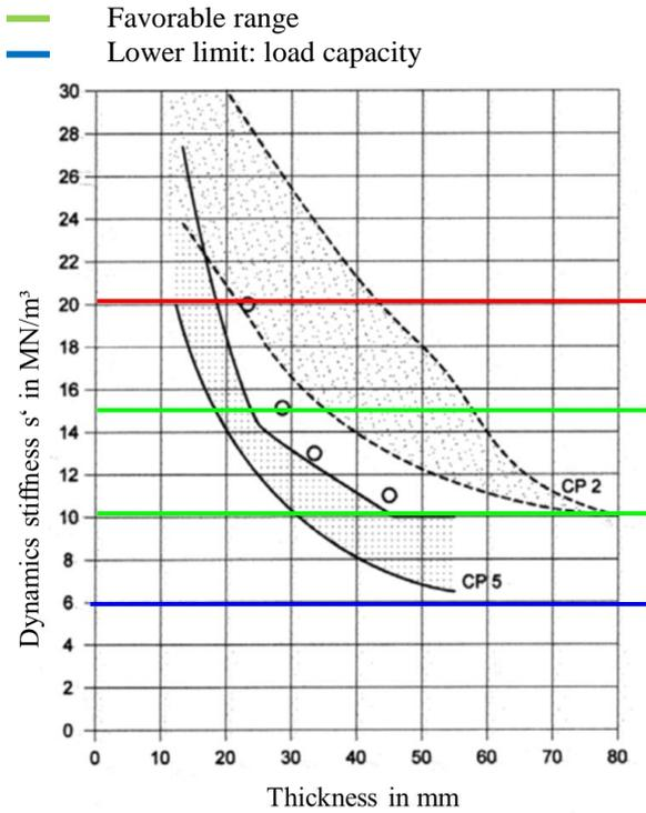
Figure 9: Dynamic stiffness of insulation layer according to OENORM B 8115-4
