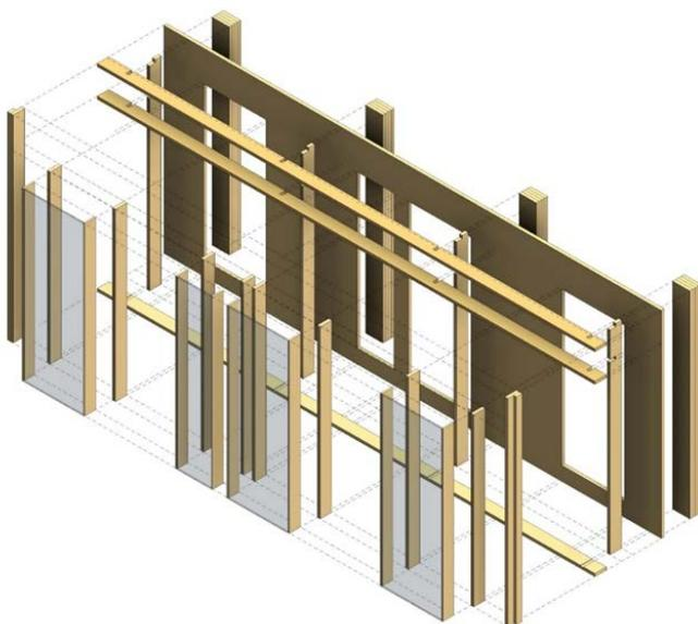
**Figure 7:** Timber-Glass façade scheme.
