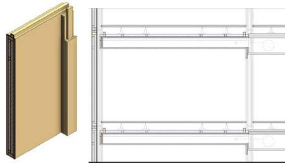
**Figure 2:** Model of a timber-frame-wall with integrated column and first approach MEP
