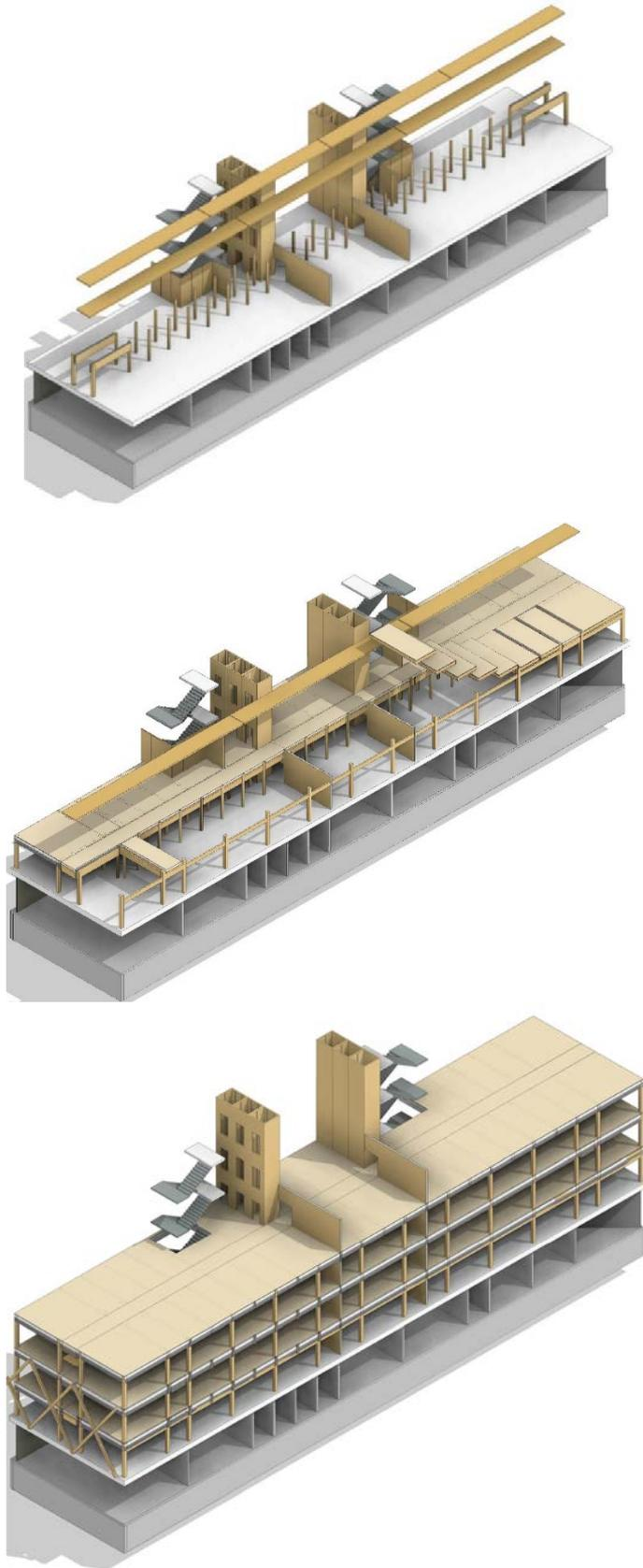
**Figure 5:** Simulation of a proposed industrialized construction process
