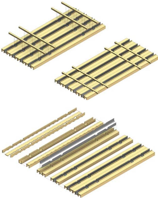
**Figure 6:** Proposal for prefabricated timber-steel-concrete-ribbed decks
