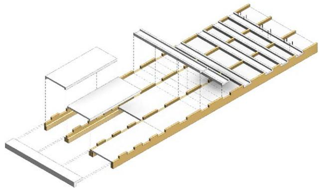
*Figure 5: Proposal for prefabricated timber-concrete-ribbed decks*
