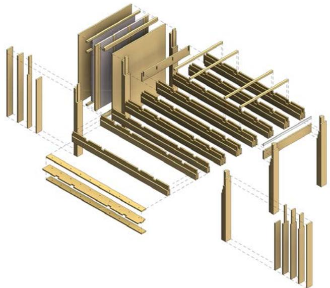
**Figure 4:** Complete system scheme including columns, walls and ribbed decks.
