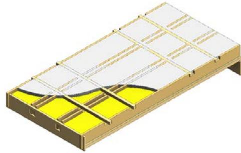
*Figure 4: Proposal for semi-prefabricated timber-concrete-ribbed decks*
