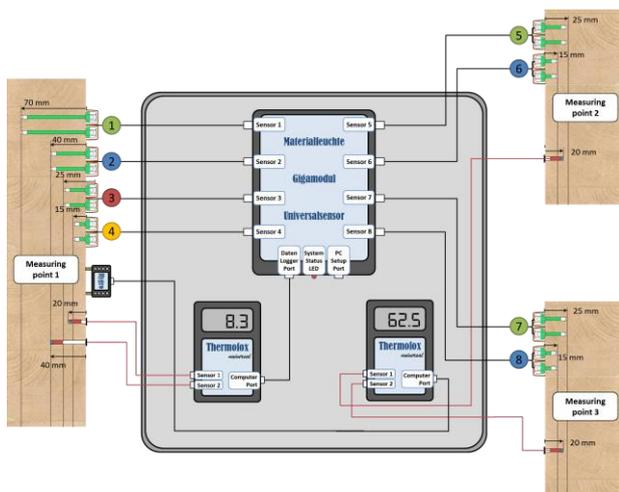
Figure 2: Schematic illustration of the measuring system
